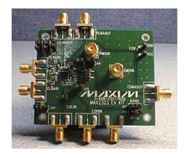
Objective: To develop and measure this dual-band triple-mode front-end IC using only 85MHz IF centers for processing PCS, cellular CDMA, and cellular AMPS.
